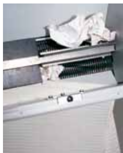
Automatic mechanical feeding system with revolving flaps
