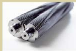
Cutters in special steel
